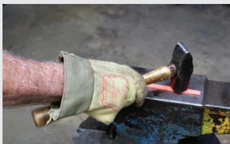
Roy hand-forges the clasp for a metal band that will fit the rim of a turned bowl.
